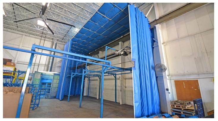
Our customer needed a three-sided retractable and stationary insulated curtain wall solution for their facility where the powder coating, drying and curing process is all conducted onsite. The induction heat used traveled throughout the warehouse which not only made it uncomfortable for the employees who were working, but also the energy inefficiency made the drying, curing and painting process take up to four days to complete the cycle.
